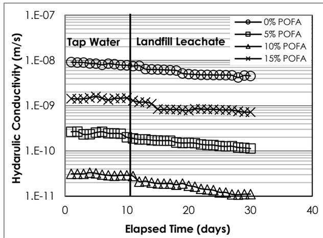
**Figure 2** Variation behaviour of hydraulic conductivity of granite residual soil – POFA mixtures with time (permeated with water and landfill leachate)
