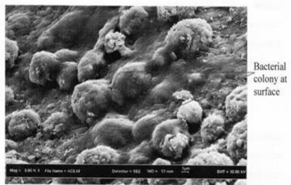
Figure 6 Bacteria immobilization on activated carbon morphology (Mag 3.0 KX)
