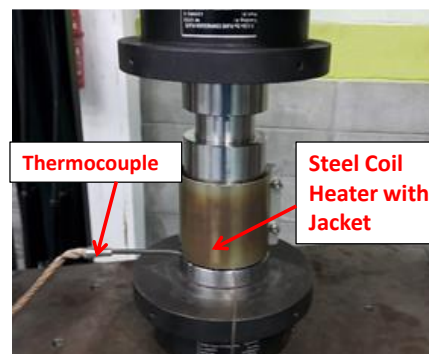
Figure 2 Briquetting process using Instron Machine 600dx
