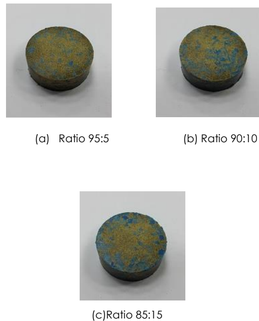
Figure 3 Image of briquettes with different mixing ratio of EFB and PE plastics
