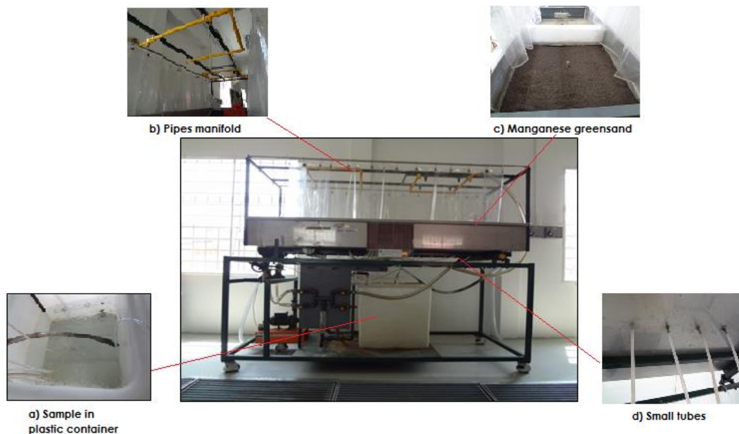
Figure 3 Equipment set-up for groundwater treatment (i.e. aeration followed by filtration) processes (a) plastic tank contained water sample, (b) pipe manifold with spray nozzles, (c) manganese greensand basin and (d) small tubes at the bottom of basin
