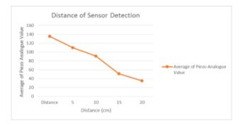
Figure 6 Graph for distance of sensor detection
