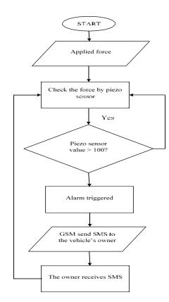
Figure 2 Process flow of Vehicle Alarm by using GSM
