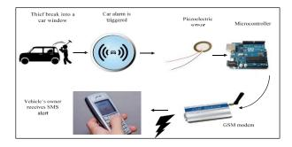
Figure 1 System Architecture Diagram
