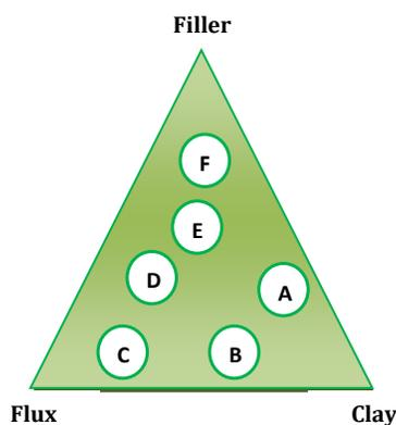
Triaxial body compositions of clay-based ceramic products
