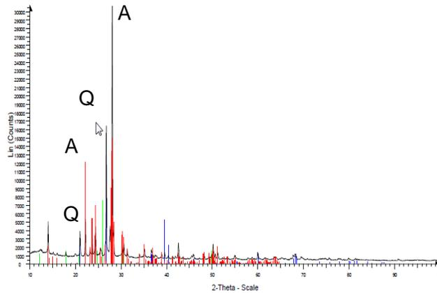
**Figure 1** X-ray diffractogram of Gua Musang Feldspar (Legend: A is Albite, Q is Quartz)
