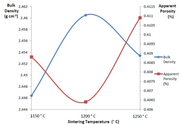
**Figure 3** Effect of firing temperature on the porosity and bulk density of a ceramic body added with GMF
