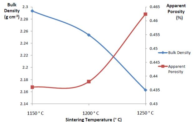
**Figure 4** Effect of firing temperature on the porosity and bulk density of a ceramic body added with GQD
