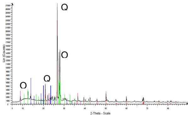
**Figure 2** X-ray diffractogram of Granite Quarry Dust (Legend: O is Orthoclase, Q is Quartz)
