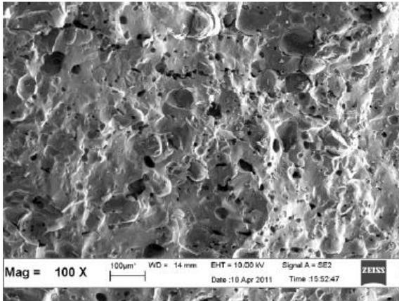
**Figure 5** Micrograph of the fracture surface of a clay body with GMF fired to 1150°C
