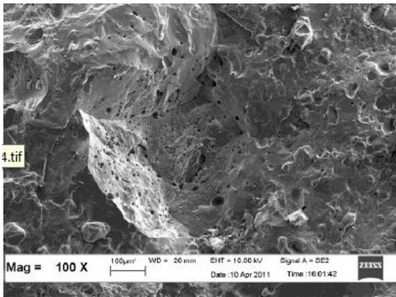
**Figure 6** Micrograph of the fracture surface of a clay body with GQD fired to 1150°C
