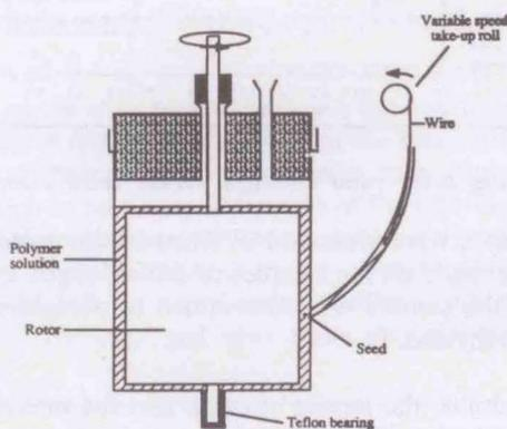
Figure 3 Schematic Diagram of the Couette Apparatus used in the surface growth method of preparing High Performance Polyethylene.
