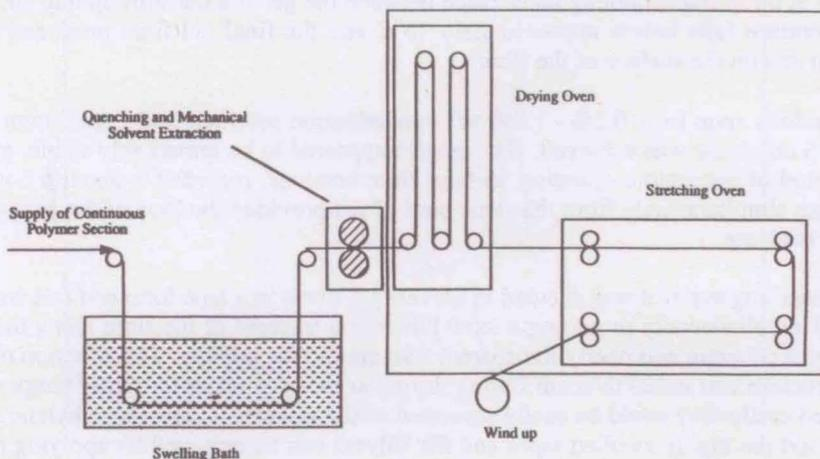
Figure 11 Schematic diagram of a swell drawing process.
