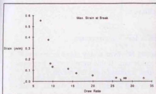
Figure 7 Maximum strain at break of Swell drawn Ultrahigh molecular weight tapes.
