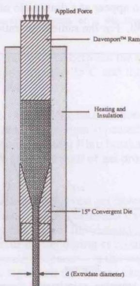
Figure 16 Schematic diagram of the ram extrusion of Gel crystallized ultrahigh molecular weight polyethylene.
