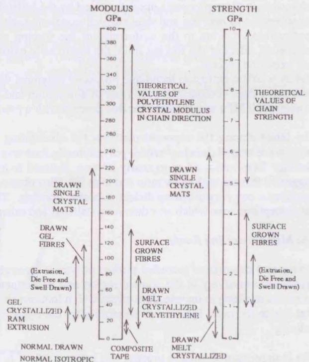
Figure 1 Development of High Performance Polyethylene Manufacturing Techniques.
