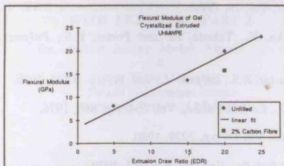
Figure 17 Flexural modulus versus extrusion draw ratio of gel crystallized ultrahigh molecular weight polyethylene extrudate (extruded at 100°C).
