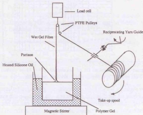
Figure 12 Schematic diagram of a die free spinning process.
