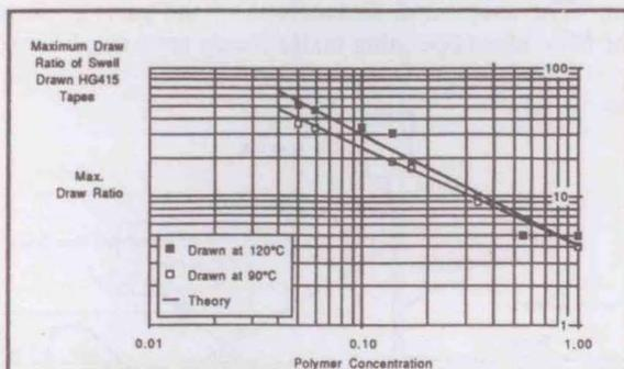
Figure 10 Theoretical fit of maximum draw ratio versus initial polymer concentration during swelling.
