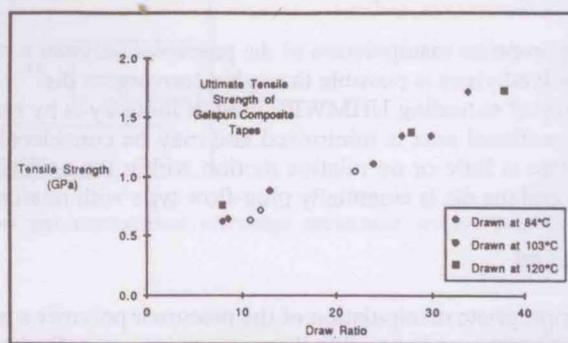
Figure 13 Young's modulus of gelspun composite tapes. Figure 14 Ultimate tensile strength of gelspun composite tape.
