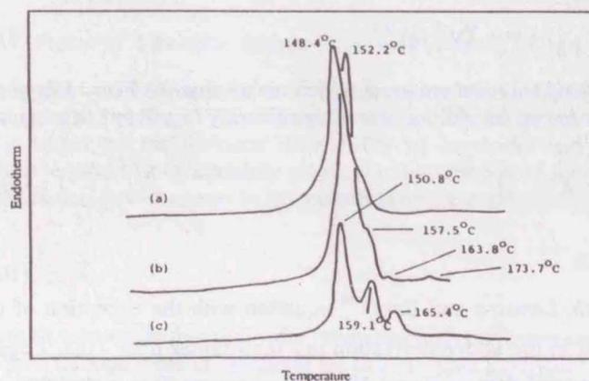
Figure 9 Differential Scanning calorimeter traces of swollen ultrahigh molecular weight tapes (conditions as in Figure 8). Draw ratio (a) 18 (b) 23 (c) 30.
