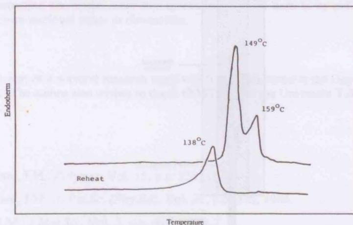
Figure 15 Differential scanning calorimeter traces of gelspun fibres. Draw ratio = 43 superimposed by the same specimen being reheated (same condition as Figure 8).
