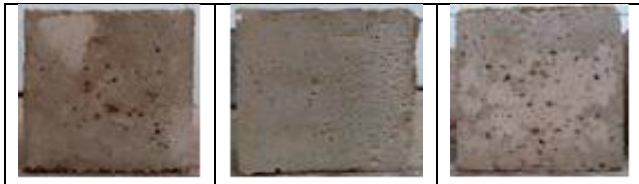
Figure 9 Surface texture of the sawdust concrete samples ratio 1:1, 1:2, 1:3 exposed to 200°C
