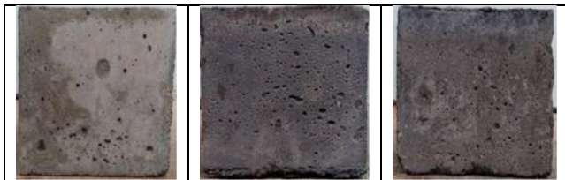
Figure 11 Surface texture of the sawdust concrete samples ratio 1:1, 1:2, 1:3 exposed to 600°C
