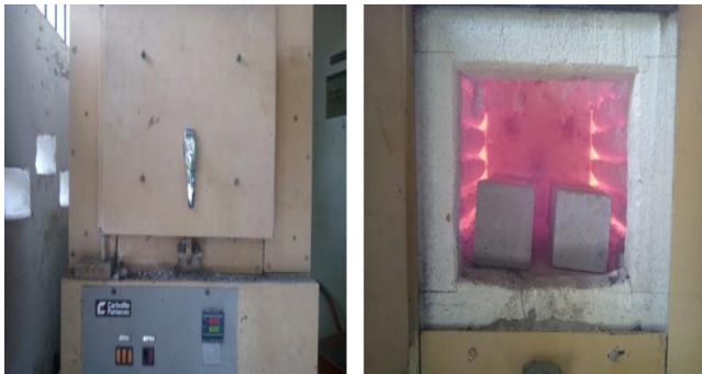
Figure 2 Electric furnace showing concrete specimens
