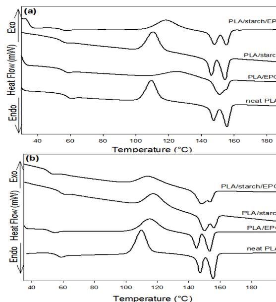
**Figure 1** DSC thermogram for neat PLA, PLA/starch, PLA/EPO, and PLA/starch/EPO blends by (a) melt blending and (b) solution casting methods.
