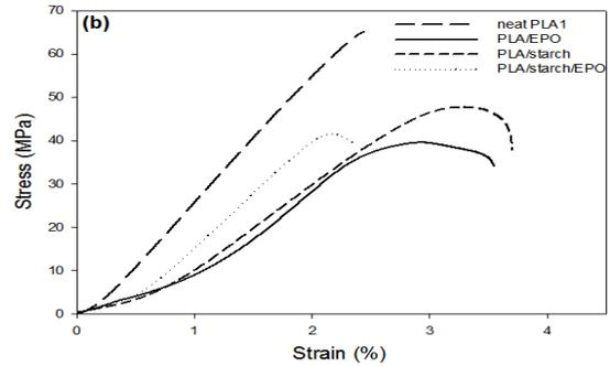
**Figure 2** Tensile strength of neat PLA, PLA/EPO, PLA/starch, PLA/starch/EPO prepared by (a) melt blending and (b) solution casting techniques.
