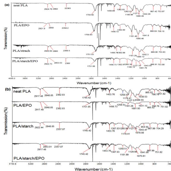
**Figure 5** FT-IR spectra for neat PLA, PLA/starch and PLA/starch/EPO prepared by (a) melt blending and (b) solution casting.
