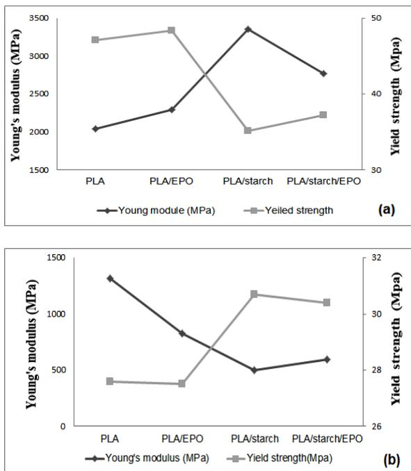
**Figure 4** Young's modulus and yield strength of neat PLA, PLA/starch and PLA/starch/EPO prepared by (a) melt blending and (b) solution casting.
