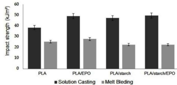
**Figure 3** Impact strength of neat PLA, PLA/EPO, PLA/starch, PLA/starch/EPO prepared by melt blending and solution casting techniques.
