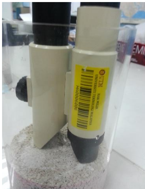
Figure 5 Soil sample surface crack width measurement
