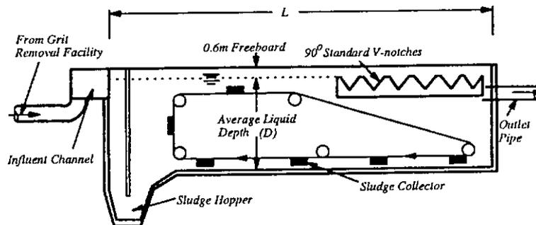
FIGURE 2: LONGITUDINAL SECTION OF PRIMARY SEDIMENTATION BASIN
