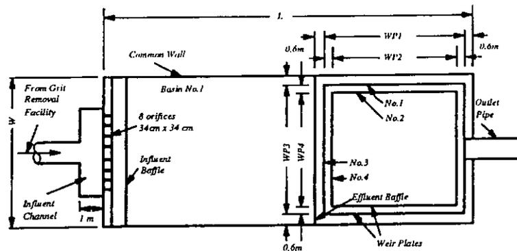
FIGURE 1: PLAN VIEW OF PRIMARY SEDIMENTATION BASIN
