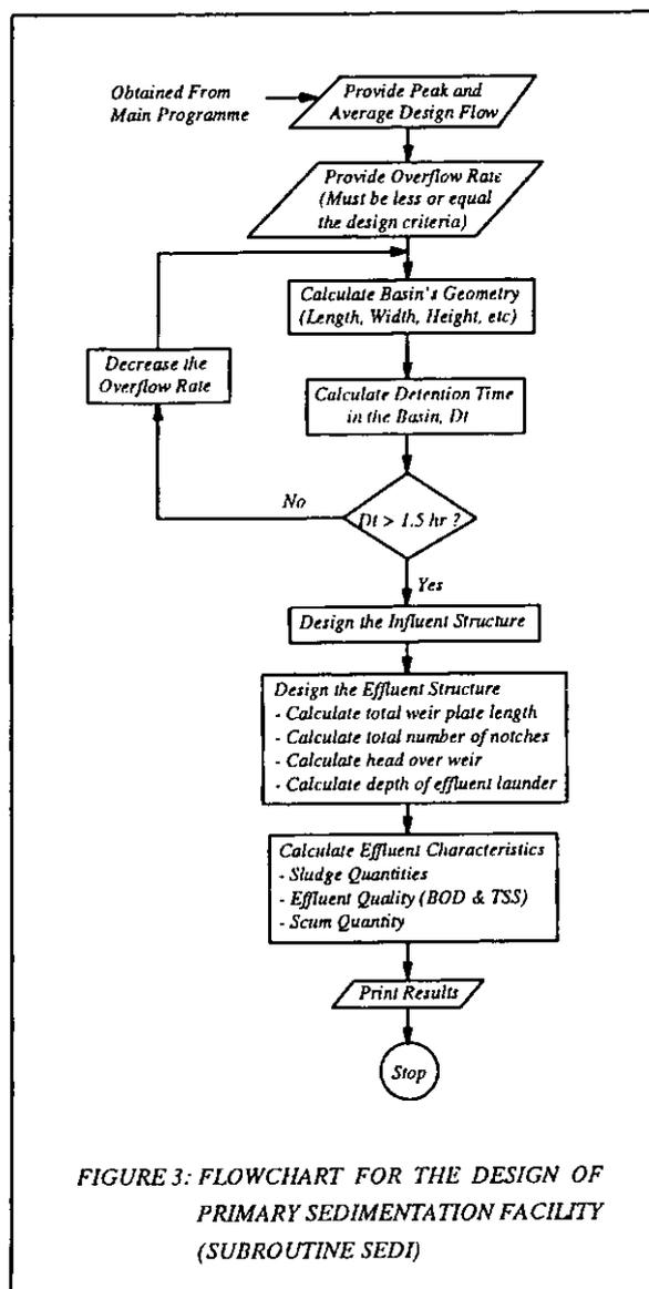
FIGURE 3: FLOWCHART FOR THE DESIGN OF
