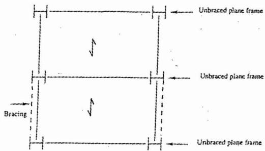
Figure 3 : Plane braced against out-of-plane sway
