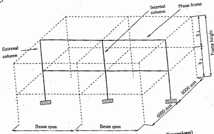
Figure 4(a): Typical layout for two bay frames (three dimensions)
