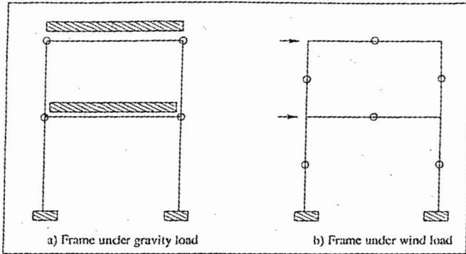
Figure 1 : Frame idealisation for "wind-moment" method
