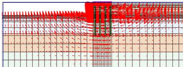
Figure 7: Displacement Vectors, (scaled up to 100 times) Case (-22, 80).
