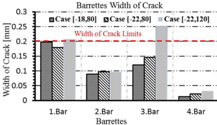
Figure 12: Width of crack for all barrettes of the diaphragm quay wall under the three studied cases.
