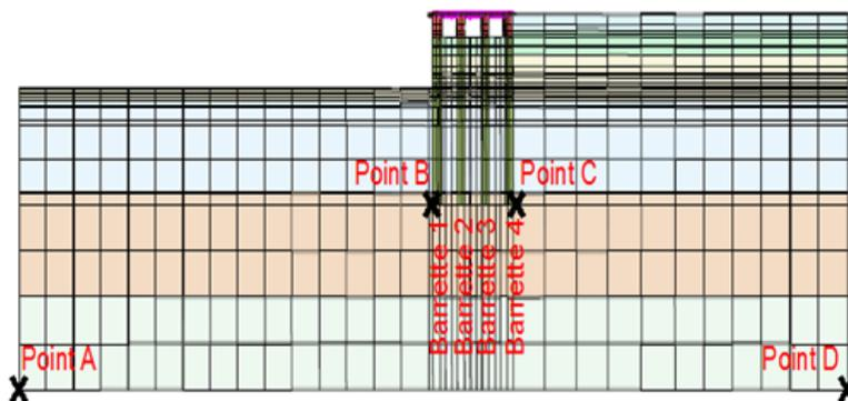
Figure 5: Finite element mesh of the quay wall.
