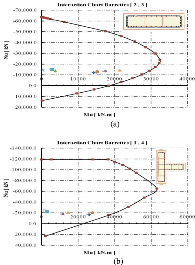
Figure 11: Interaction diagrams for barrettes (a) For barrettes 1 and 4, (b) For barrettes 2 and 3.
