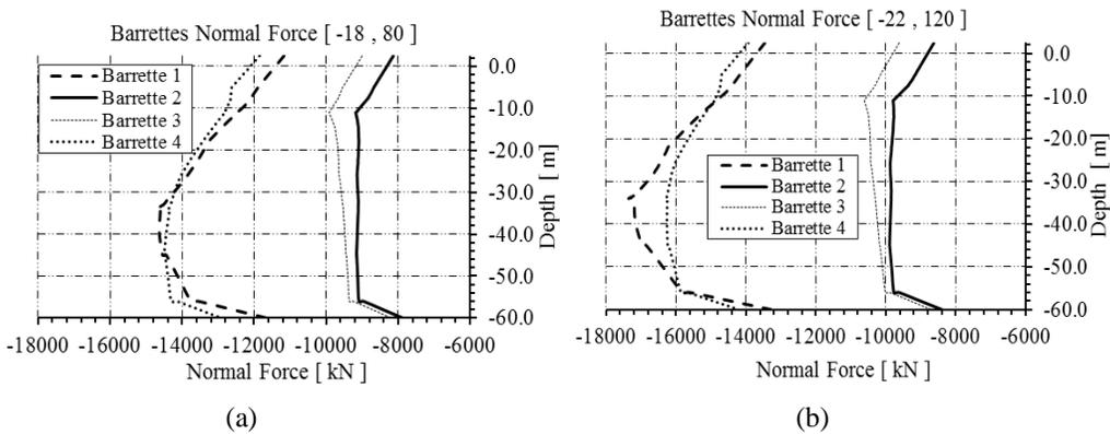
Figure 10: Normal force, (Axial force) for barrettes (a) Existing Case (-18, 80), (b) Second scenario of development case of (-22, 120).
