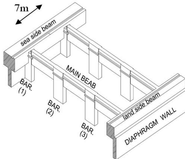
Figure 3: Quay Wall beams alignment
