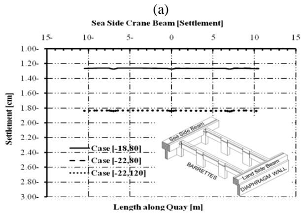
Figure 13: Vertical settlement of crane beams (a) Sea side crane beam, (b) Land side crane beam.
