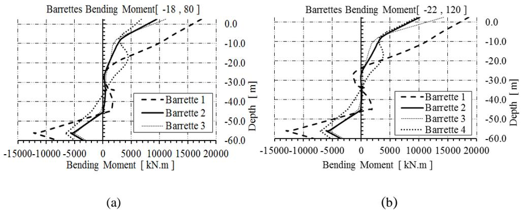
Figure 9: Bending moment for barrettes (a) Existing Case (-18, 80), (b) Second scenario of development case of (-22, 120).
