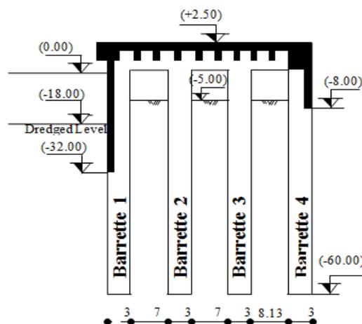
Figure 2: Quay Wall cross section (all dimensions in m.)
