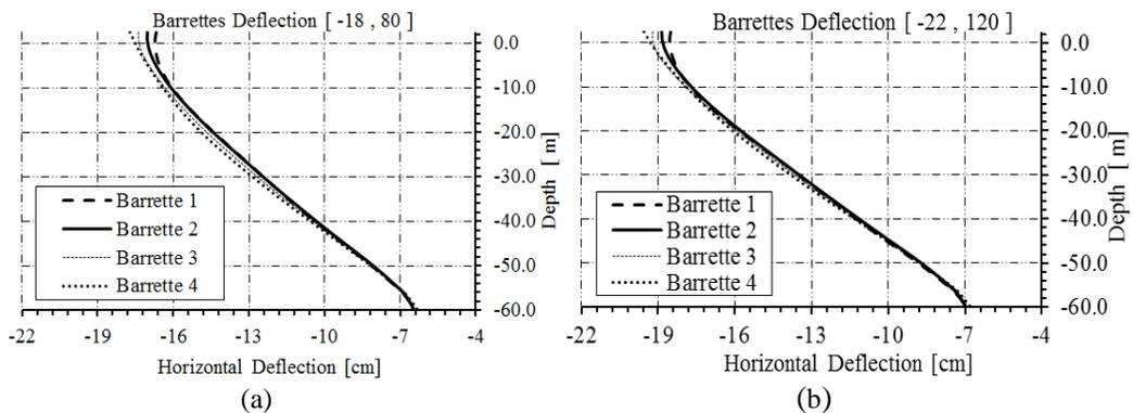
Figure 8: Horizontal deflection for barrettes (a) Existing Case (-18, 80), (b) Second scenario of development case of (-22,120).
