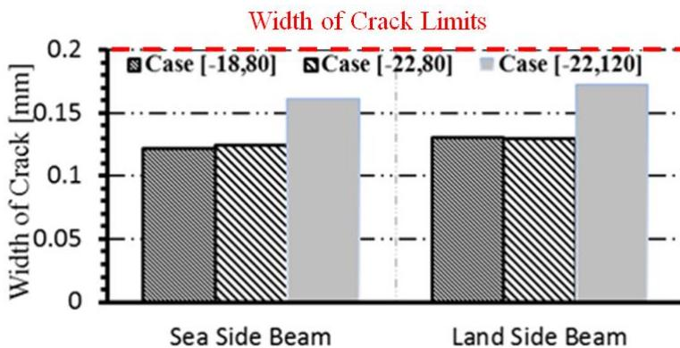
Figure 15: Width of crack for sea side and land side crane beams under the three studied cases.
