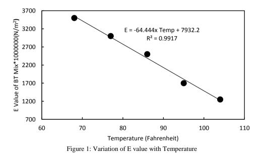
Regression equation may be used to interpolate / extrapolate the E Value to other temperatures. This paper presents pavement design based on seasonal variation and
