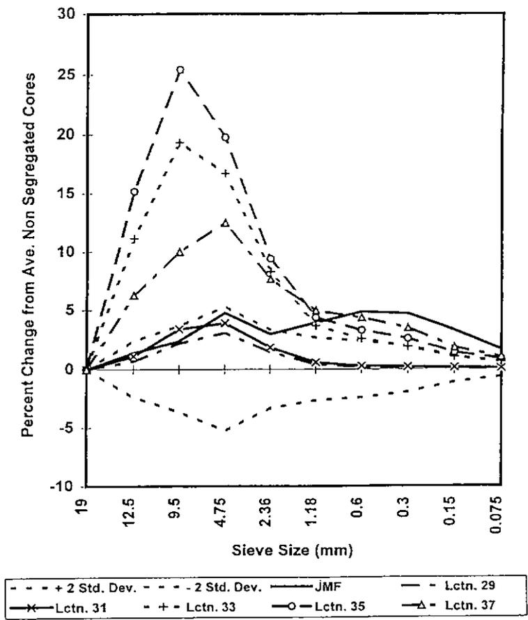
**Figure 1** Variation in gradation for segregated cores compared to the average gradation of the non-segregated cores for site 2.
