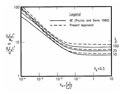
Figure 3 : Normalized Head Deflection (or Rotation) Response for Free-Head Pile
