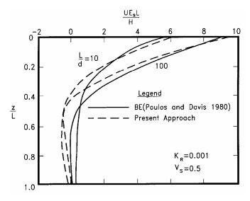
**Figure 5 :** Deflection Profile Along Free-Head Pile
