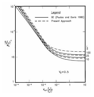
Figure 4 : Normalized Head Rotation Response for Free-Head Pile
