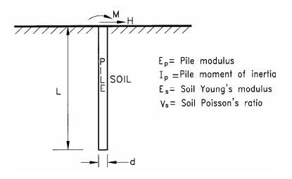
Figure 1 : Definition of Laterally Loaded Pile Problem
