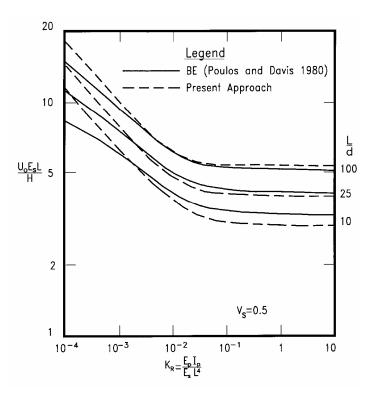
Figure 2 : Normalized Head Deflection Response for Free-Head Pile
