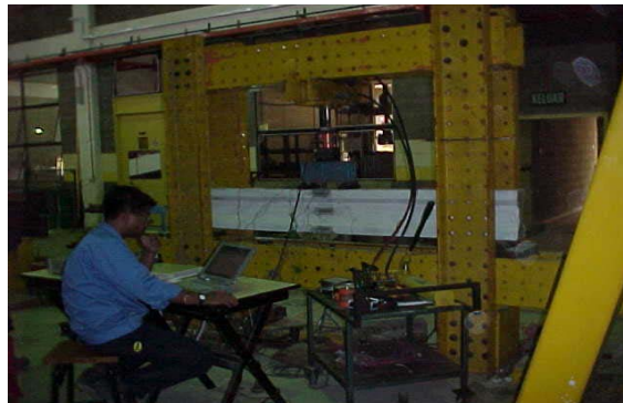
Figure 2: Two Point Load Test on Prestressed Lightweight Concrete Beam
