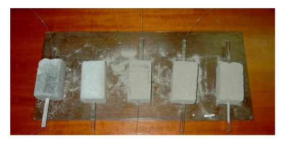
Figure 1: Samples of reinforced mortar prisms
