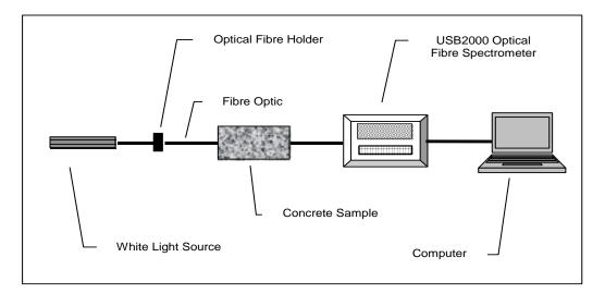
Figure 4: The illustration of experimental Setup
