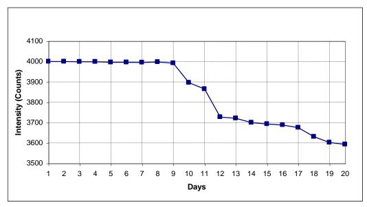
Figure 7: Intensity count against days of Sample B immersed in 10% NaCl solution
