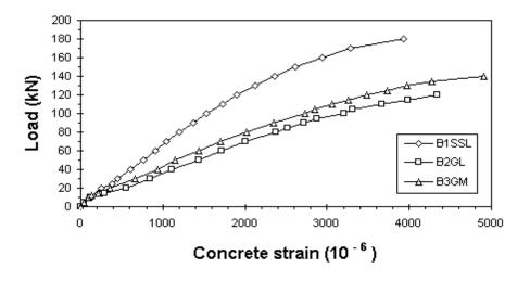
Figure 3: Load-concrete strain for all the beams tested
