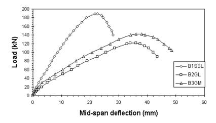
Figure 2: Load-deflection of all beams tested
