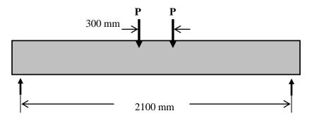
Figure 1: Schematic diagram of the test set-up
