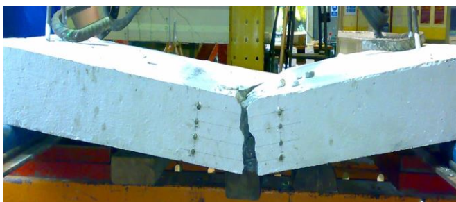
Figure 9: Failure mode of plain concrete slab (SC-PLAIN)
