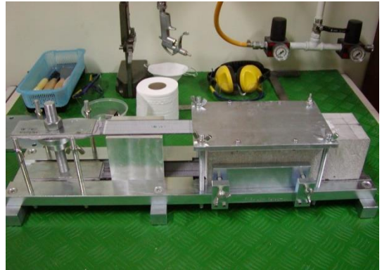
Figure 8: Jig used for proper bonding
