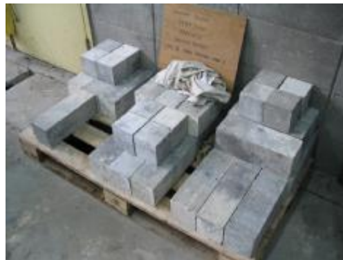
Figure 2: Concrete prisms left for curing
