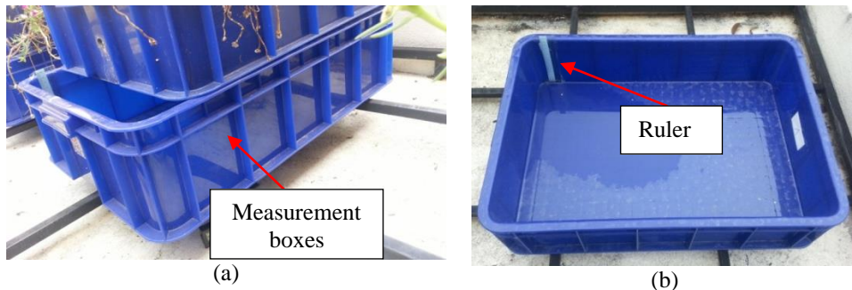
Figure 2: (a) Measurement box under one of the green roof plot (b) Example of measurement box with the ruler for height measurement
