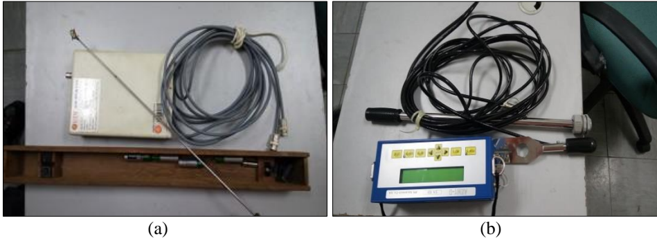
Figure 6: Flow calibration; (a) a miniature velocity, and (b) an Electromagnetic Flow Meter (EFM).
