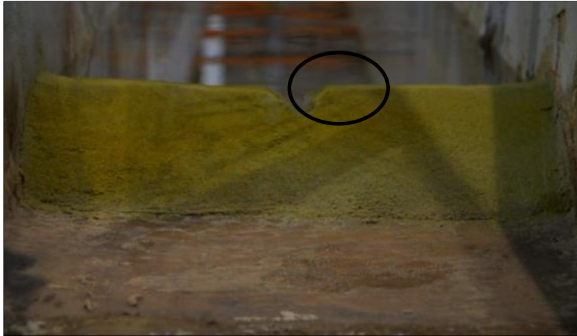
Figure 9: A notch; acting as a weak point of the embankment dam, is located at the middle of the embankment filled.
