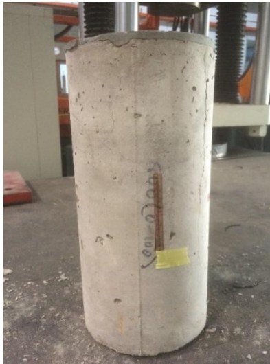
Figure 4: Cylinder specimen completed with the capping material and strain gauges
