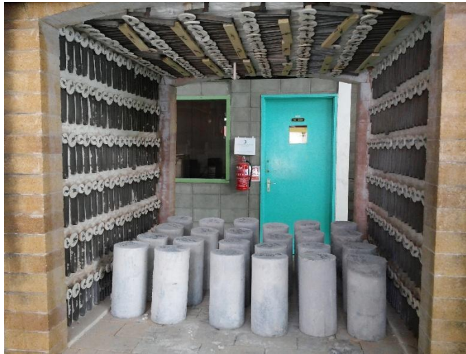
Figure 3: Firing furnace for the elevated temperature exposure
