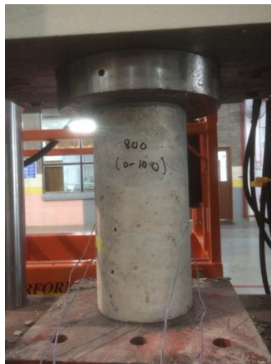
Figure 5: Test setup for the Elastic Modulus and compression load
