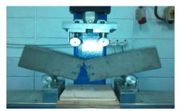
Figure 2: Broken prism sample after flexural test
