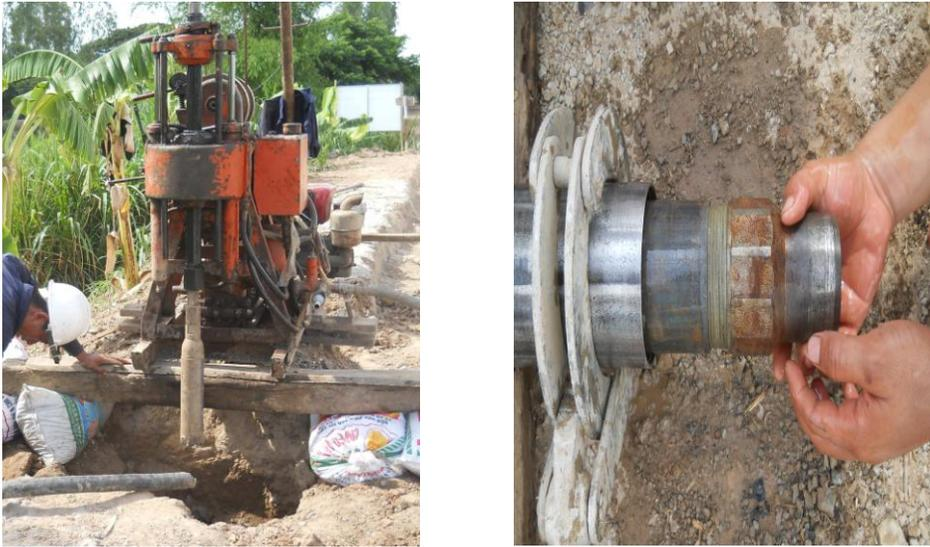
Figure 6: A XY-100 drill machine and a double Shelby tube used to take core samples at the field
