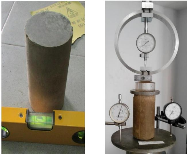
Figure 8: A soilcrete specimen made and a UCS test setup on the TSZ30-2.0 triaxial instrument in the laboratory according to ASTM D-2166, ASTM D-1633, and TCVN 9403:2012.
