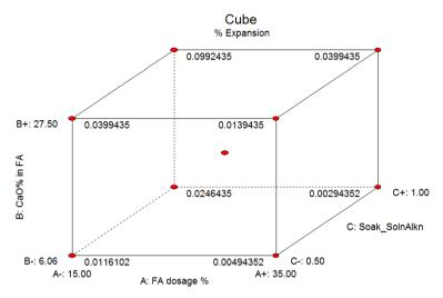
Figure 3: Cube plot of factorial design for FA dosage, CaO% of Fly Ash and Soak Solution Alkalinity effects with expansion values.
