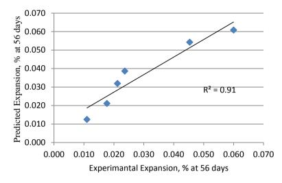
Figure 7: Correlation between experimental and predicted values of six different fly ashes at 56 days.
