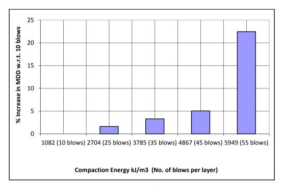
Figure 2: Graph of Compaction Energy (kJ/m<sup>3</sup>) v/s Percentage Increase in MDD
