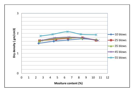
Figure 1: Graph of Moisture content v/s Dry Density at varying number of blows per layer
