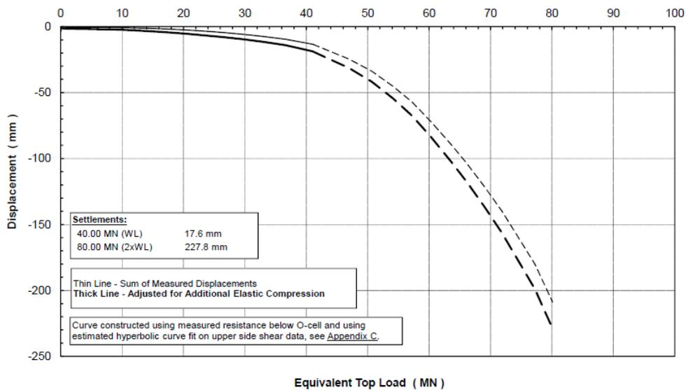
Figure 8: Equivalent Load Settlement Curve
