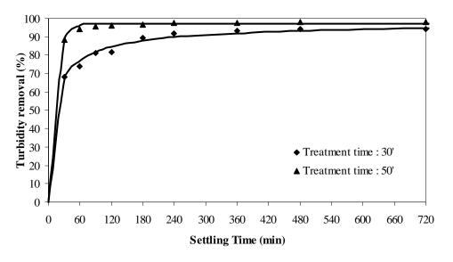
Figure 5: Effect of EC time on turbidity removal at DC of 0.8 A
