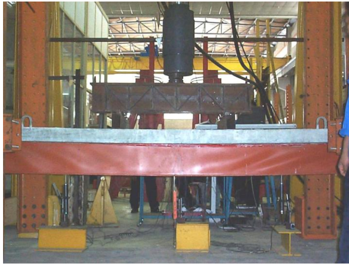
Figure 12 : Failure of flat web composite beam specimen due to global web buckling
