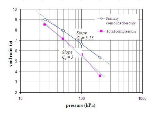
Figure 8: Typical e-log p' curve for determination of compression index
