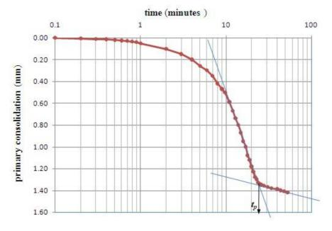
Figure 6 : Time-compression curve for primary consolidation only
