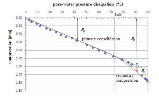
Figure 5: Typical compression-degree of consolidation curve from consolidation test
