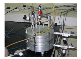
Figure 2: Rowe consolidation cell used in this study
