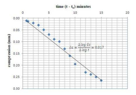
Figure 7 : Determination of index of secondary consolidation ( $\delta_a$ )
