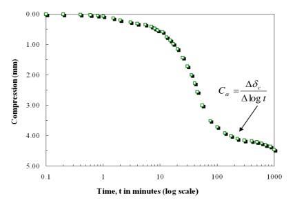
Figure 3: Typical time compression curve from consolidation test
