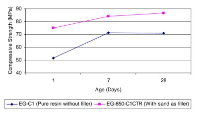
Figure 1: Compressive strength of epoxy cubes (without filler) and epoxy cubes (with filler) at various ages
