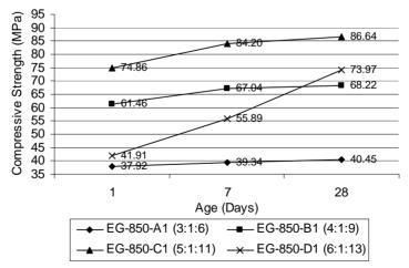
Figure 2: Compressive strength of epoxy grout with different epoxy: hardener: filler ratios at various ages
