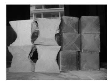
Figure 4: Failure mode of epoxy grout compared to cement grout after compressive strength test
