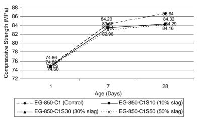
Figure 3: Compressive strength of epoxy grout with various replacement level of GGBFS as filler (epoxy:harderner:filler ratio 5:1:11)
