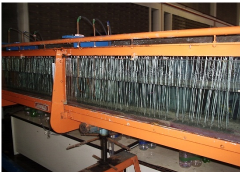
Figure 2: Side and plan views of experimental set-up for estuary with resisting structures (case 3). Concrete slabs with the embedment of steel wires acting as resisting structures (shown on the left)
