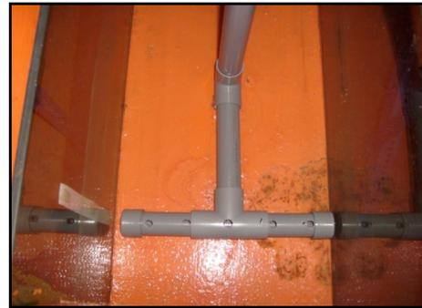
Figure 2: Multi-port diffuser pipe in cross-flow direction
