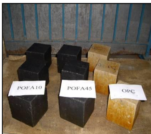
Figure 4: Specimens after exposure to acid solution
