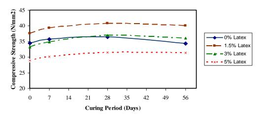
Figure 1: Effect of latex dosage on compressive strength
