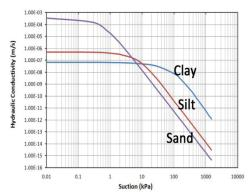
Figure 3:Typical hydraulic conductivity curve for soil
