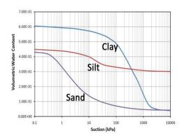
Figure 2:Typical SWCC curve for soil
