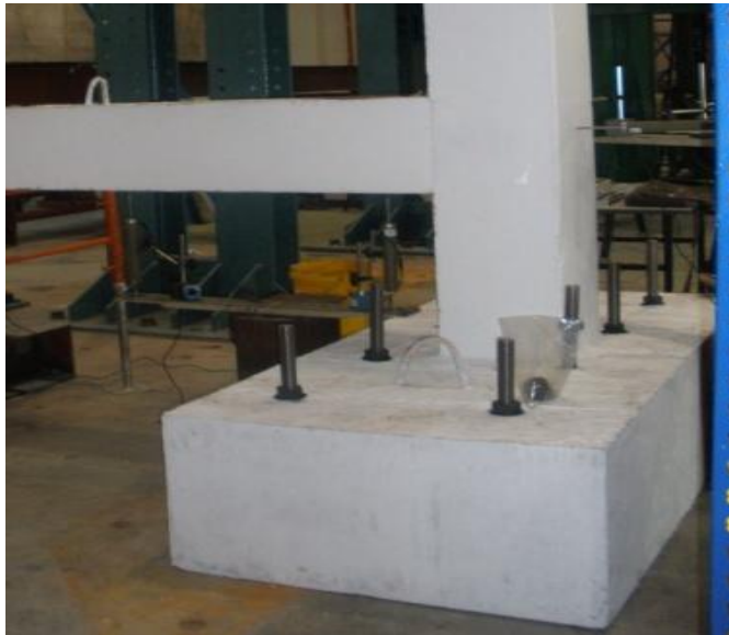
Figure 13: Foundation beam is clamped to strong floor using high-yield threaded rod.
