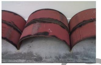
Figure 1 : Original X70 pipe segments
