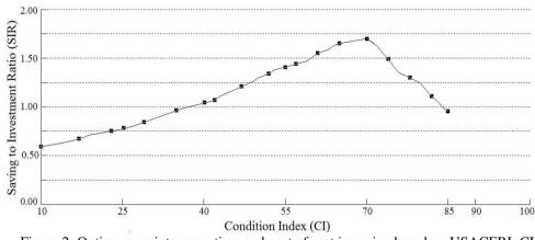
Figure 2: Optimum maintenance time and cost of cast iron pipe based on USACERL CI
