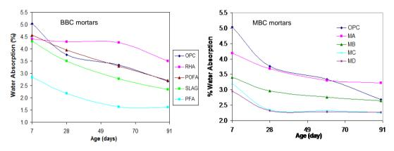
Figure 1: Water absorption of BBC and MBC mortars
