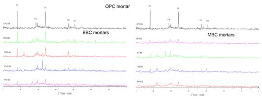
Figure 5: XRD patterns for OPC, BBC and MBC mortars
