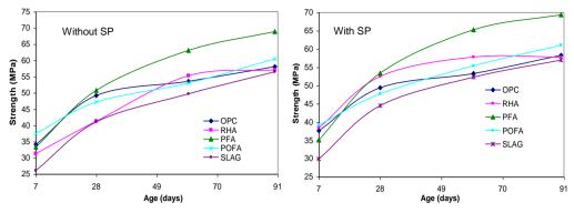
Figure 3: Compressive strength of BBC mortars at different age
