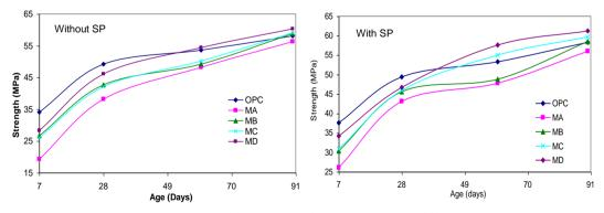
Figure 4: Compressive strength of MBC mortars at different age
