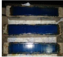
Figure 2(h) Beam specimens after strengthening
