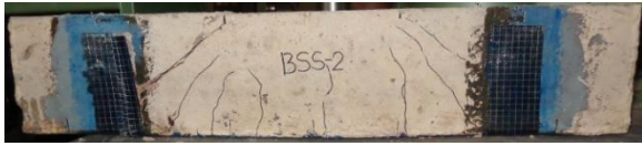
Figure 10 Ultimate failure of BSS-2 with flexural-shear crack formation
