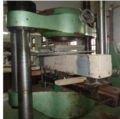
Figure 4(c) Test setup of beam
