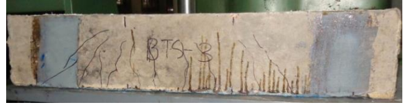
Figure 8 Beam specimens BTS-3 with after ultimate failure
