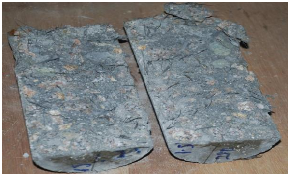
Figure 7: Distribution of steel fibre in broken cylinder.
