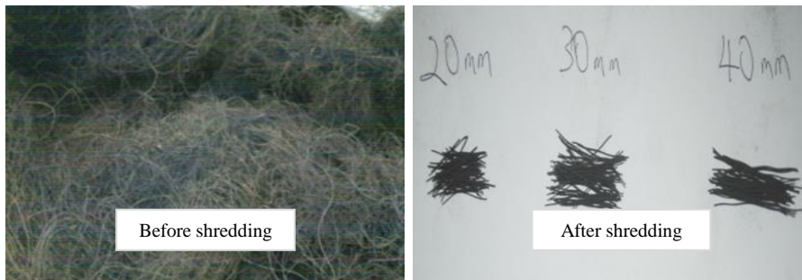
Figure 1: Recycled steel fibre before and after shredding
