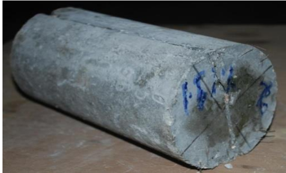
Figure 6: Concrete cylinder after splitting tensile test.
