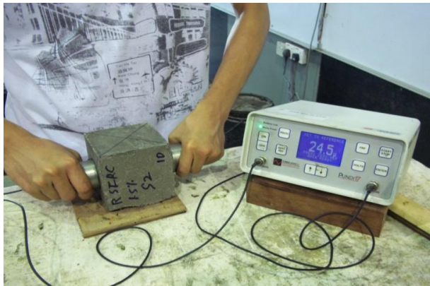
Figure 2: Testing of ultrasonic pulse velocity.
