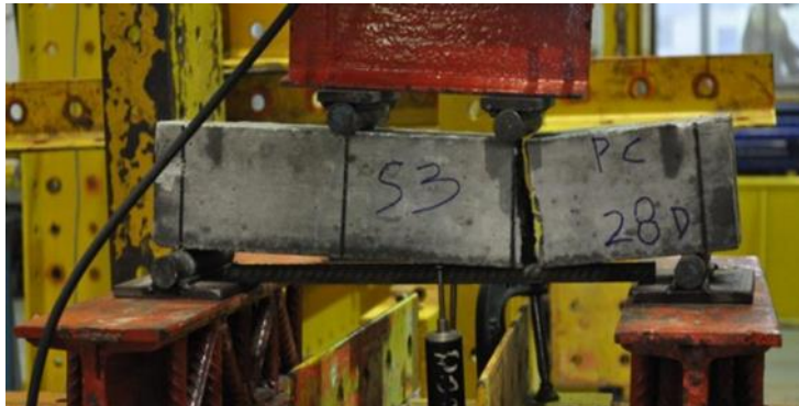
Figure 8: Failure mode of plain concrete beam in flexure.
