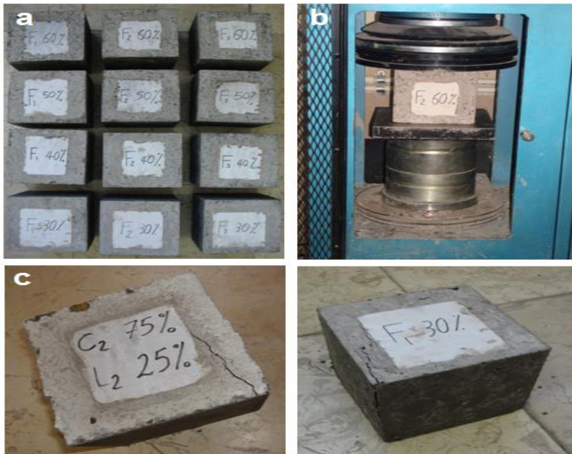
Figure 5: (a, b, c) Testing compressive strength of concrete specimens: (a) specimens before testing, (b) Loading of specimens, (c) after testing.
