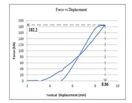
Figure 7: Axial Force vs Vertical Displacement for Sample 2- Bridgestone
