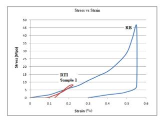
Figure 12: Compression Test and Comparison of RTI (sample 1) and RB sample (Turer and Ozden, 2008)
