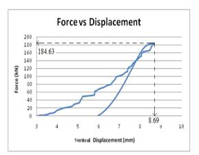
Figure 11: Axial Force versus Vertical Displacement for Sample 4-Falken
