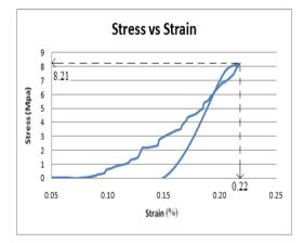
Figure 10: Stress versus Strain for Sample 4 - Falken
