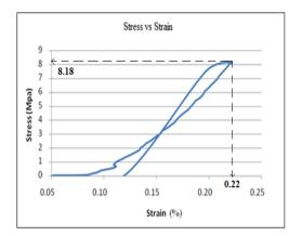
Figure 4: Stress vs Strain for Sample 1 - Bridgestone
