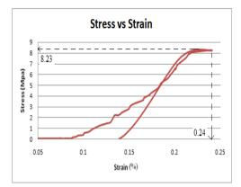
Figure 8: Stress versus Strain for Sample 2 - Dunlop
