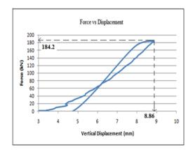
Figure 5: Axial Force vs Vertical Displacement for Sample 1- Bridgestone
