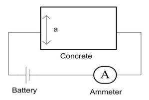
Figure 4: Basic Measure Resistivity
