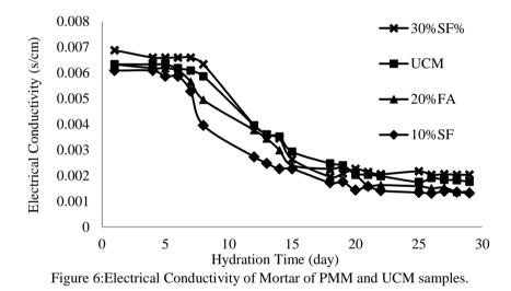
It can be observed that 10% SF has the lowest conductivity in comparison to 20%FA, 30%SF and UCM. 30%SF has the highest conductivity which is reflected on its worst EI. This is due to the increase in ionic concentrations and mobility of these ions as more water exists within the pores. PT, SCM and ECT results were in correlation with CS test results as the mechanical property of samples.
