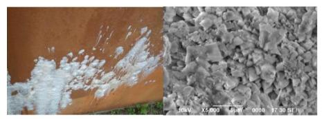
Figure 1:(a) Efflorescence on concrete wall (b) Scanning Electron Micrograph (SEM) image of efflorescence collected from the wall.
