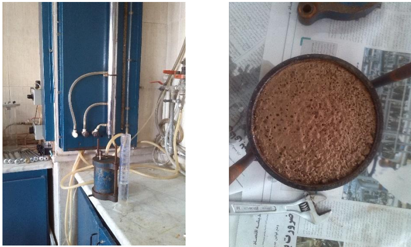
Figure 2: The cell used for soil leaching (left) and sample G2 after leaching (right)
