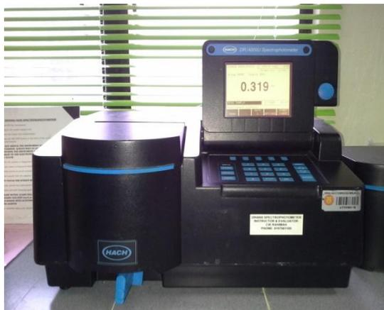
Figure 2: Spectrophotometer DR4000 used for the study.
