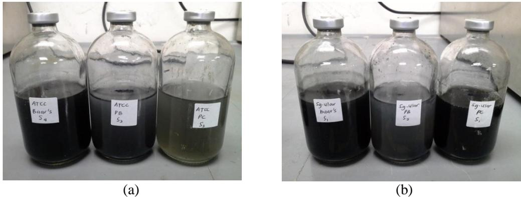
Figure 1: Sulphate-Reducing bacteria in Modified Baar's, Postgate B and Postgate C. a) ATCC 7757. b) SRB isolated from site.
